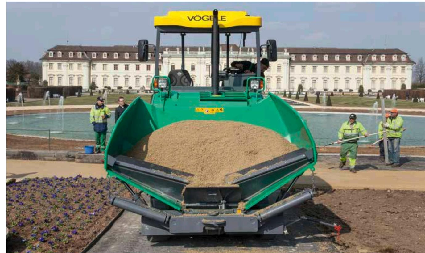
Despite the paver's slim profile, its material hopper holds 10t. The hydraulic hopper front (option) supports both supply of the paver with mix and emptying of the material hopper. The paver comes with oscillating push-rollers to ensure the shock-free docking of feed vehicles.
