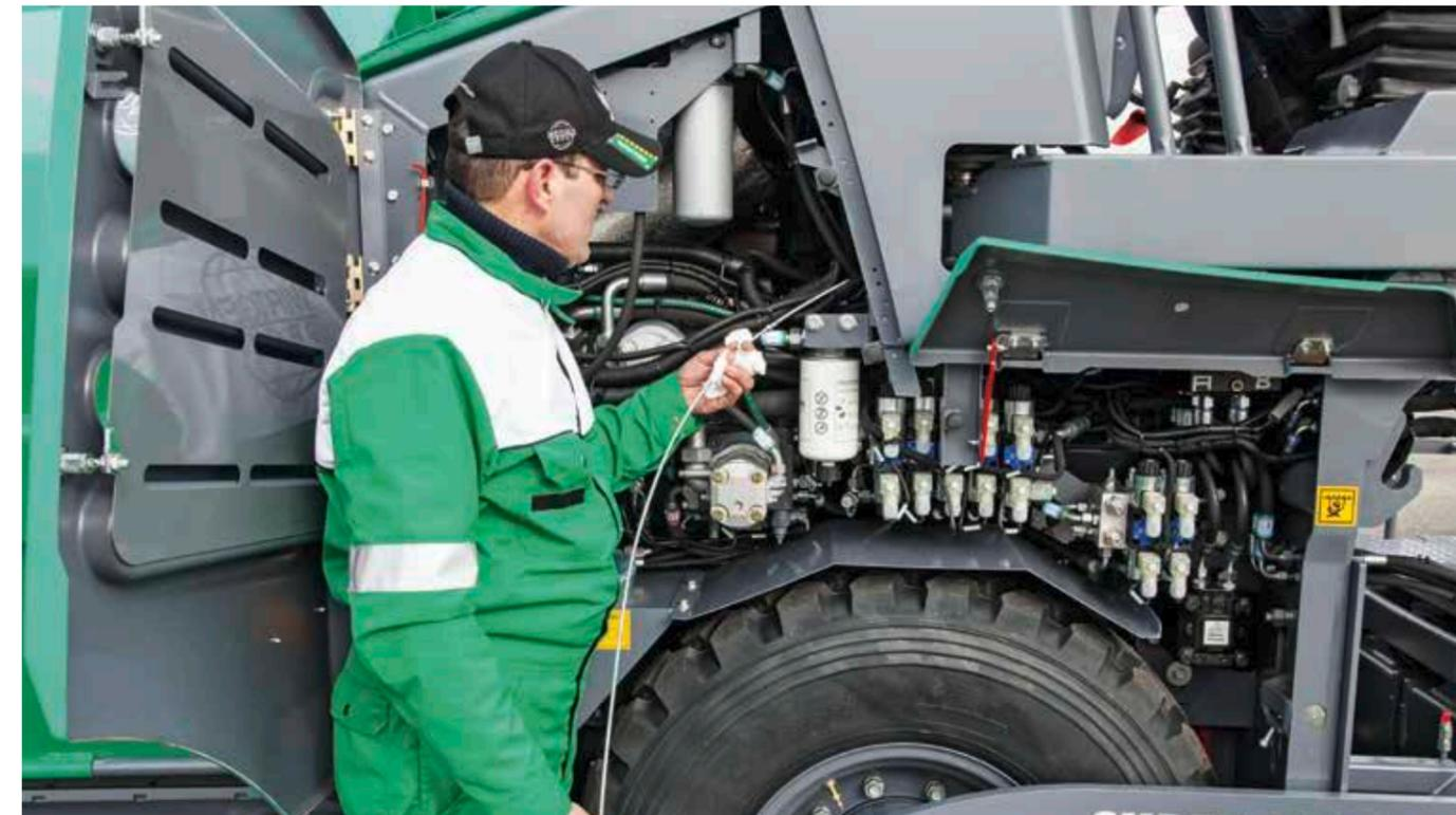
The identical servicing concept of the "Dash 3" pavers permits rapid, uncomplicated maintenance. All servicing points on the machine are easily accessible via large hinged panels.
