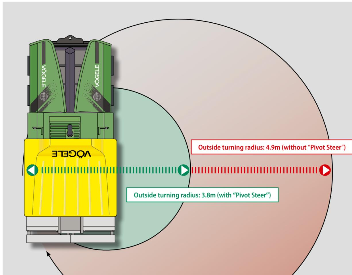
The "Pivot Steer" steering brake reduces the torque of the rear inner wheel on "Dash 3" pavers, enabling them to turn almost on the spot and reducing the outside turning radius to as little as 3.8m.
