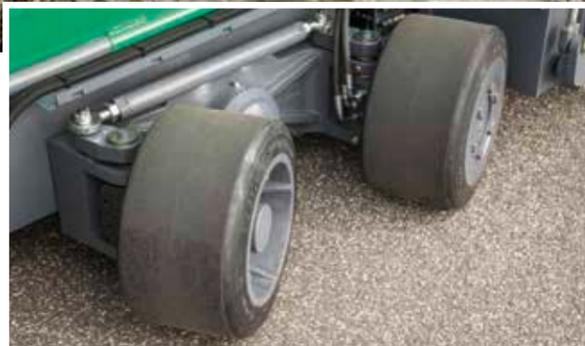
A powerful paver that's a comfortable drive on the road. The precise steering and handling characteristics make for the SUPER 1303-3i's excellent manoeuvrability, as demonstrated by its outside turning radius of just 4.9m (3.8m with "Pivot Steer"). With its powerful traction drive, the machine can pave swiftly and travel on public roads at a maximum speed of 20km/h. So if its next job site is close at hand, there is no need for a low-bed trailer to transport the paver.
