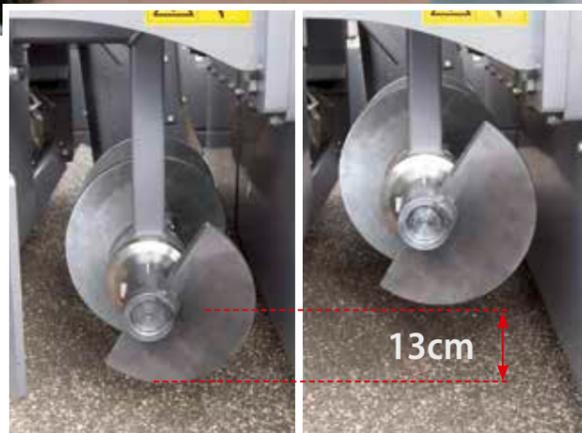
The conveyance and spreading of mix in front of the screed is optimal thanks to the large conveyor tunnel, proportional control of conveyors and powerful augers. Furthermore, augers adjustable in height and folding limiting plates for the auger tunnel allow the paver to be moved on the job site without a need for conversion. This saves time and money.
