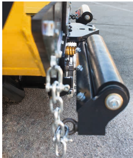
Impact-free docking – dampened bumper.
