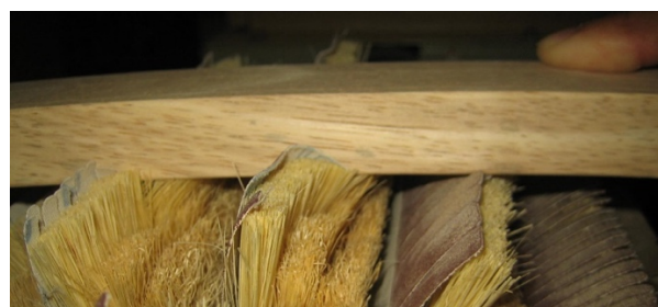
Figure 15: Excessive penetration with sharp abrasives
