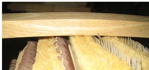
Figure 14: Proper depth, with sharp abrasives
