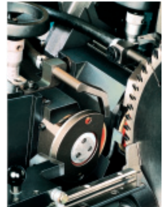
Measurement device for compensation of grinding wheel wear as an optional extra.
