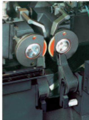
The stable blade clamp can be opened wide to simplify saw blade changeover.
