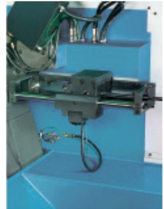
The Vollmer saw blade retainer guarantees precision centering and trouble-free saw blade changeover.
