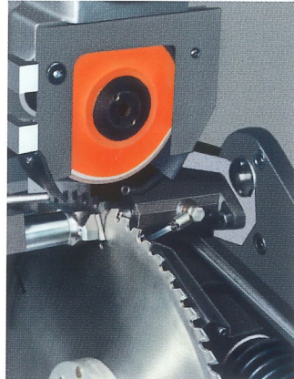
Stable blade clamping eases changing the saw blade.
