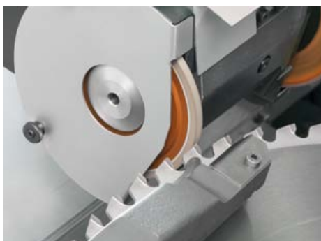
Clearance surface processing with left spindle nose.
