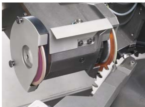
Hook surface processing with combi grinding wheel.
