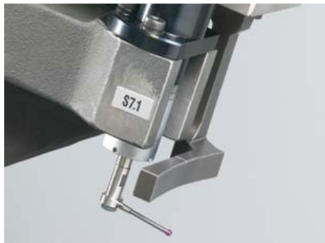
Automatic data collection by means of the measuring probe.
