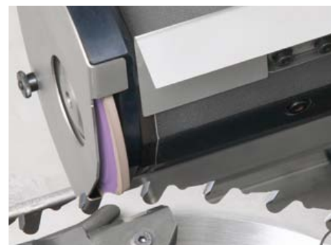
Tool body processing with CBN grinding wheel.
