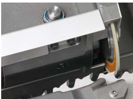
Clearance surface processing with combi grinding wheel.
