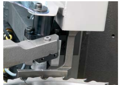
Saw stop for the precise positioning of the saw blade.
