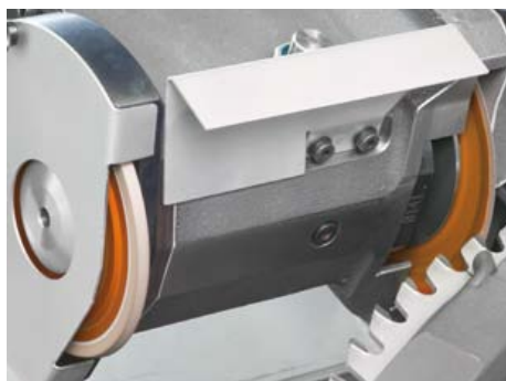
Hook surface processing with right spindle nose.
