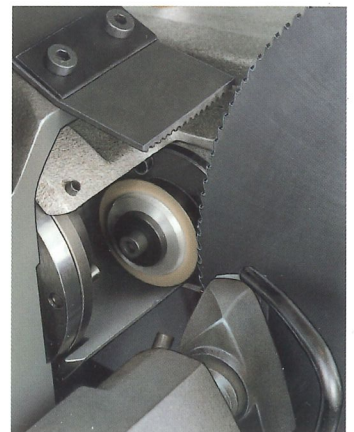
Option: grinding of a chip breaker groove for small tooth pitches from 7 mm
