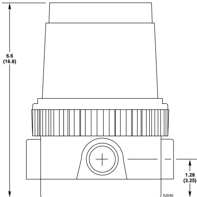
Figure 1—Dimensions of DCU Enclosure in Inches (Centimeters)
