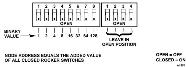
Figure 3—Field Device Address Switches
