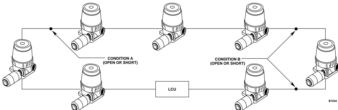
Figure 2—Communication by means of the Digital Highway
