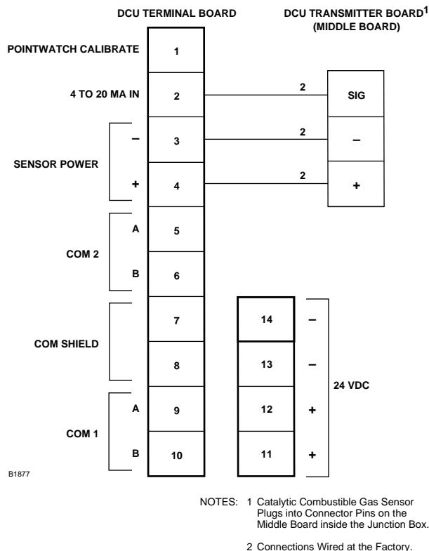
Figure 9—DCU Transmitter Board Connected to Terminal Wiring Board
