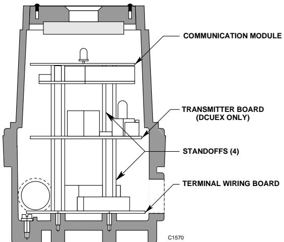
Figure 8—Printed Circuit Boards in Combustible Gas DCUEX
