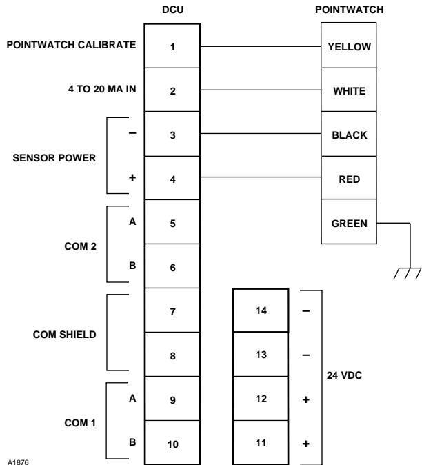
Figure 7—PointWatch Connected to DCU
