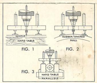
(Show example of how plastometer is placed under sample)
