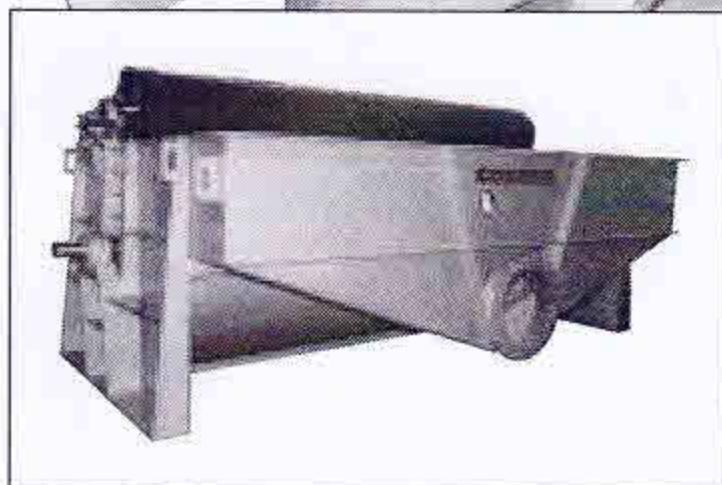
The Free-Flo Thickener is used to thicken stock from ~0.7-1.0% up to 6% consistency, depending on the furnish. Available in a 60-in. mold diameter with mold faces from 48 to 234 inches, it has unit capacities ranging from 20 to 400 T/D. Applications include thickening in OCC and board mills, as well as washing in ONP and ledger grade deinking systems. It can also be used as the primary thickener ahead of a belt or screw press in a kneading or dispersion operation.
