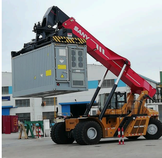
Figure 4-3 Top lifting by four points vertical crane
