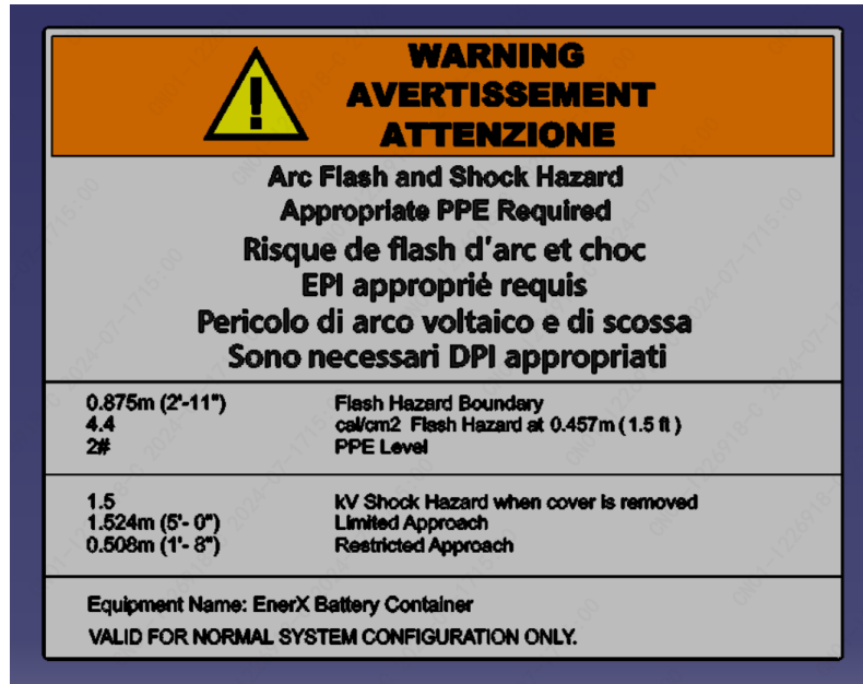
Figure 1-2 Arc Flash Label
