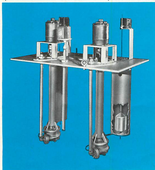
Sump pumps in duplex unit have float switches shown with special stilling columns and high water alarm
