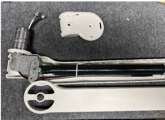
Figure 16: Preparing LCH Spring Arm with Camera - Cover Removal
