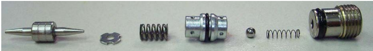
Figure 9-2: One side of inside components of pilot check valve of rotary valve
