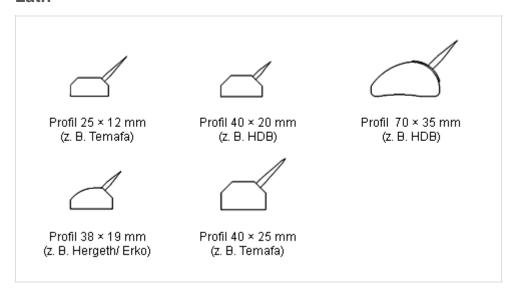
Under normal conditions, beech laths are adequately stable. Massive laminated laths should be chosen if the work load is heavier. The spiked lath profile depends upon the chosen pins.
