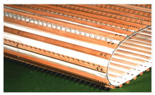
Our standard spiked lattices consist of beech or laminated beech laths which are screwed or riveted on belts. This construction method allows for infinite variety so that the appropriate spiked lattice can be constructed for each machine.
