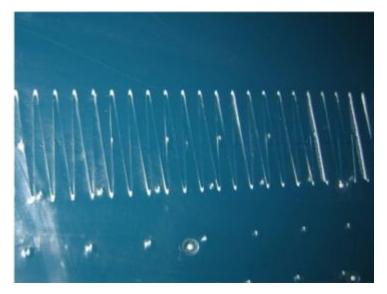
The same applies to the other belts in terms of durability. For the endless connection, the belt has finger formed and layered cut-outs. The layers are then overlapped and welded together i. e. joined together by melting the material. Upon request, the belt ends can also be cut at a slant and then welded. This enables the endless connection to be spread over a greater length.
