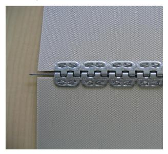
If the Transition belt cannot be installed in the machine endlessly, a hinge connection should be chosen. Two hinge-type metal strips are attached to the belt ends and the endless connection formed by inserting a wire.
