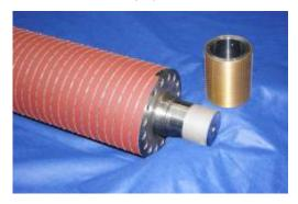
Our biggest spiked rollers are more than 4 m long. Therefore only a cut-out of them can be presented to you. These spiked rollers are solid steel rollers with pins and they have got a friction lining. Such huge spiked rollers are used to transport carpets out of carpet weaving machines. Due to the existing high loads theses rollers consist of only one shaft.
