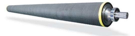
Needle rollers System "GEVA" are in similar dimesions. These transport-rollers are steel-rollers covered with plastic and coated with a friction pad. The pins are hammered into the surface. They are used in weaving machines of Dornier, Picanol/Meersschaerdt or Itema/Sulzer. Because the pins are set from outside they can be replaced easy. The friction pad cannot be replaced.
