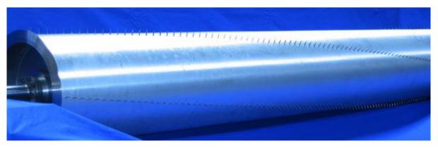
The last example shows a pinned roller for textile machines. In opening machines fibres are hold back by help of such rollers. High roller speeds and beating loads make a precise and safe production process necessary.
