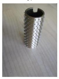
The spiked rollers of the opposite picture are used in wood processing machines. In edge gluing machines it is necessary to transport the edge to be glued safely within the machine. Our proven spiked rollers with a diameter of for example about 20 mm always perform this task excellently.
