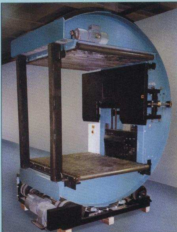
The center axis style inverters are ideal for automated line installations and can be fitted with power roller conveyors on the base and platen.
