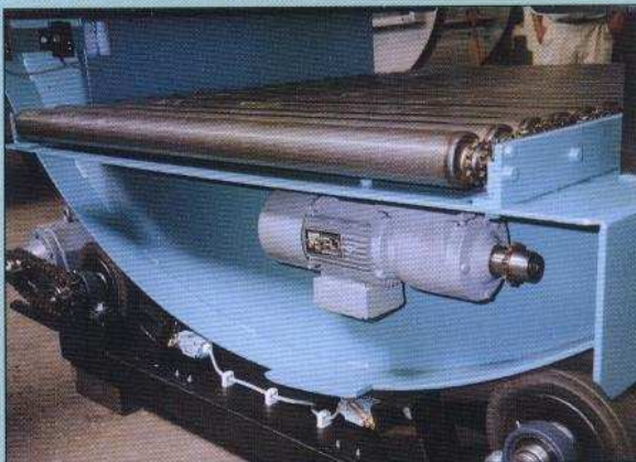
The center axis style inverters are ideal for automated line installations and can be fitted with power roller conveyors on the base and platen.
