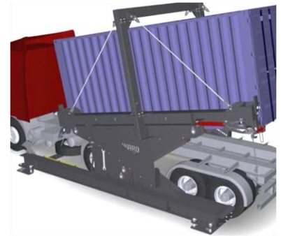
Fig.22: Tilt container up to align the rear swinglocks
