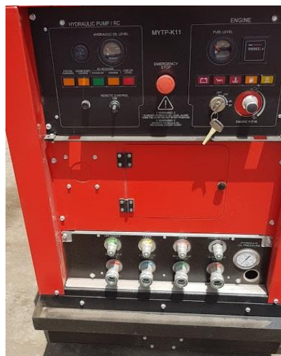
Fig.10: Colour coded hydraulic hoses
