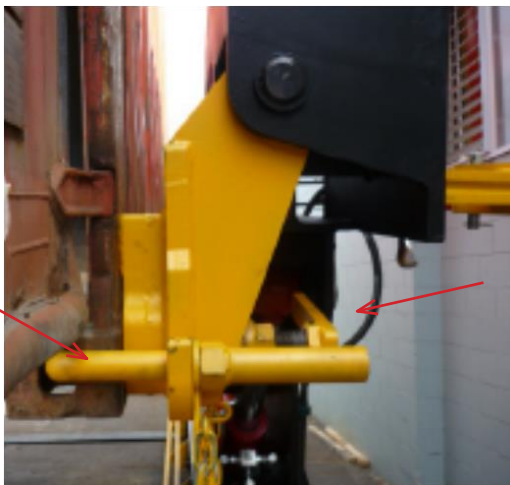
Fig.21: twistlock and "J" hook secured
