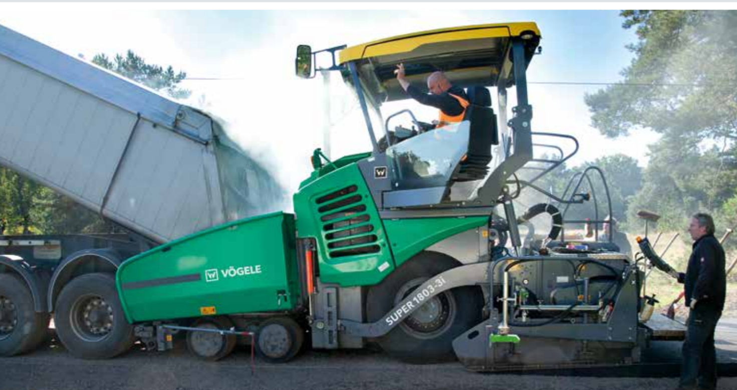
The power unit of the SUPER 1803-3i with diesel oxidation catalyst (DOC) and selective catalytic reduction (SCR) for exhaust gas after-treatment complies with the strict requirements of European exhaust emissions standard Stage 4 and US EPA standard Tier 4f.
