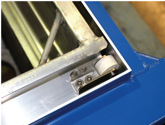
3.4g Roller Jack Roller at Discharge End
