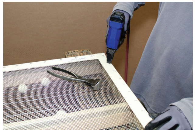
3.21 Screen Installation on General-Purpose Screen Frame
