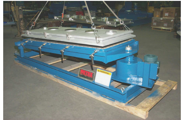
3.1 Top cover removal using lifting hooks and overhead hoist
