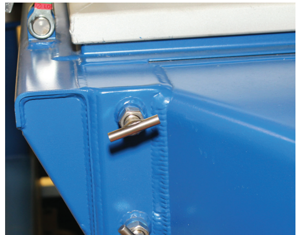
3.5 Screen Frame Jacks at Feed End of Screen Box Assembly
