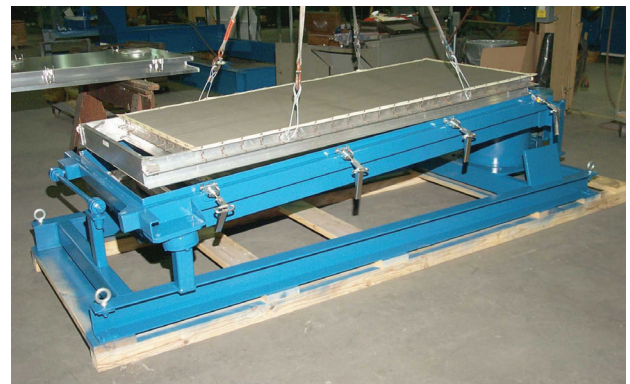
3.2 Lifting the Screen Frame
