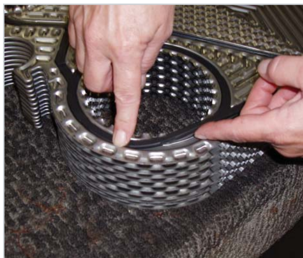
Lock-in gaskets speed the assembly process. They can be replaced during shutdown — saving you time and money.
