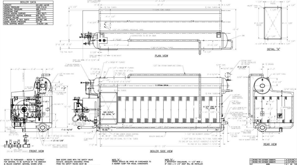
THIS DRAWING NOT INCLUDED IN THE CONTRACT WILL NOT BE SUPPLIED WITHOUT SUPPLEMENTARY AGREEMENT, MATERIAL NOT SUPPLIED BY B&W WILL BE DULY NOTED. B&W SCOPE ENDS WITH 8" SCH80 BW OUTLET FOR CONNECTION TO STEAM LINE, WEIGHT
