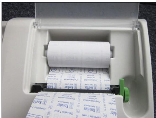
Figure 42 Printer - change of thermal paper
