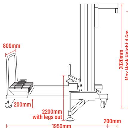
Note 1: Counterweights must be secured before lifting.
