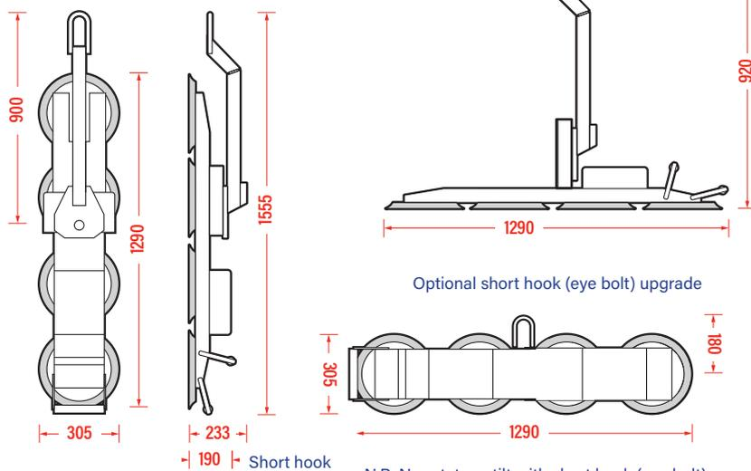
N.B. No rotate or tilt with short hook (eye bolt)
