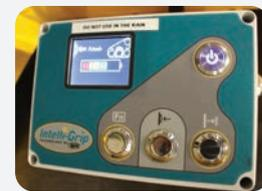
The Intelli-Grip technology on the MT2 monitors the vacuum lifter in real-time.
