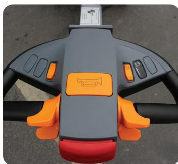
Drive backwards and forwards and the raise/lower function is controlled from the ergonomic control lever with built-in emergency stop.
