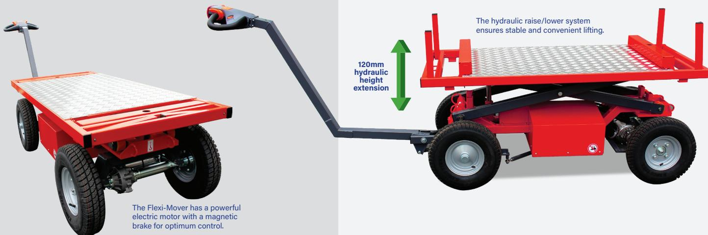
The Flexi-Mover has a powerful electric motor with a magnetic brake for optimum control.
