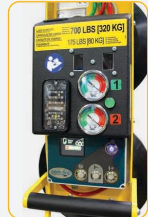
The Intelli-Grip technology monitors vacuum lifters in real-time.
