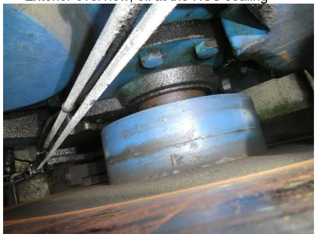
Exterior overview, oil at the HSS sealing
