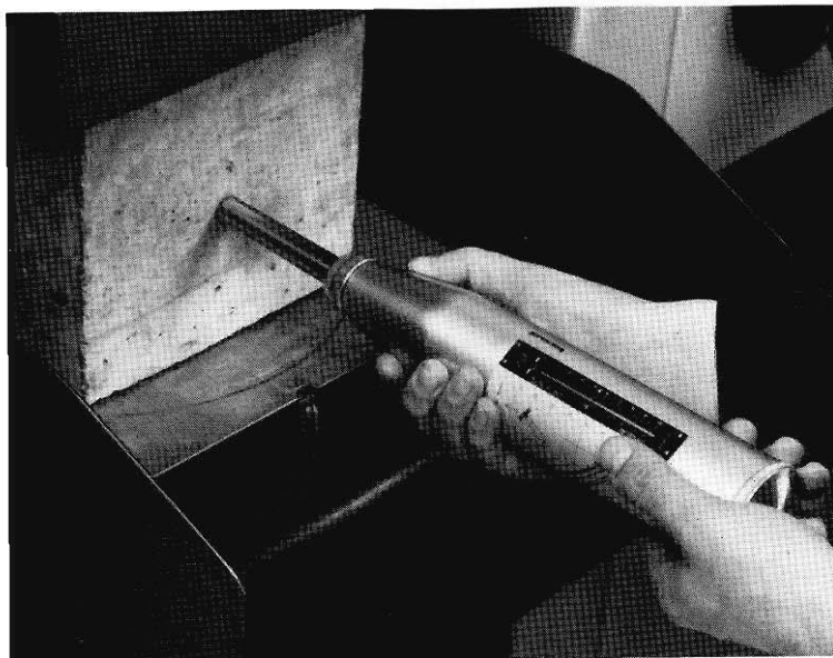
Fig. 1 The Concrete Test Hammer Type L during Calibration Tests carried out in the Swiss Federal Institute for Testing Materials in Zurich, Switzerland
