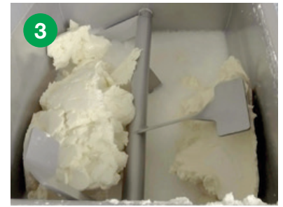
After 20 minutes, the buttermilk is secreted and discharged through the outlet valve.
