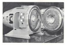
Hinged end housing—Disk access is a hinged end-housing containing the adjusting mechanism and sliding head assembly. Electrical conduit to the gearmotor has sufficient slack to permit the head to swing without disconnecting terminals. Plates shown are the segmental type—although one-piece plates are available.
