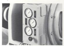
Rotor lock—A patented device which automatically prevents axial movement of the rotor during startup and shutdown.
