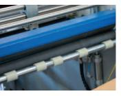
The adjustable burster automatically separates sheets up to B2 size.
