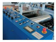
The centralised PLC control panel offers ease of operation and is enhanced with a modem link for remote diagnostics.
