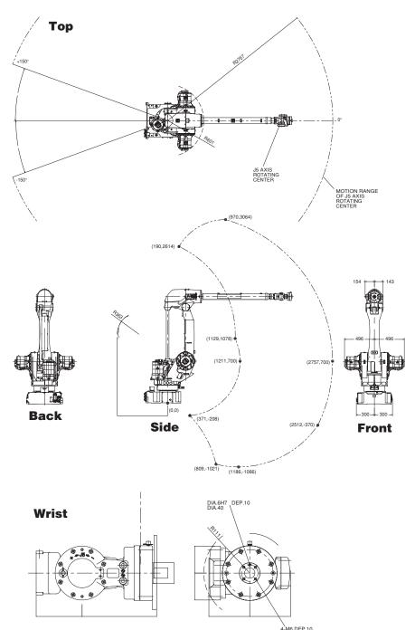
**Note:** Dimensions are shown in millimeters. Detailed CAD data are available upon request.
