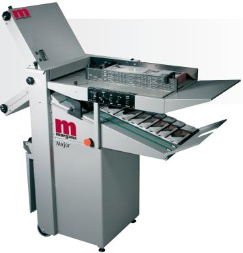
enter the fold plates. The feed table also has a suction chamber to control curled or statically charged paper.
