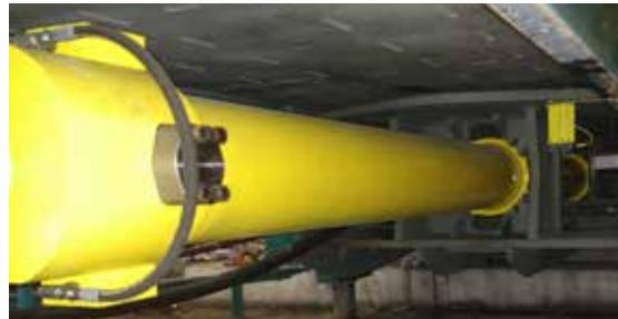
11" main-ram cylinder with up to 427,649 lbs. of platen force delivers up to 30% more force than competitive balers using 11" cylinders.
