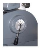
The roller nip adjustment quickselect notch system used on the RSC-1401CLTW roll laminator significantly simplifies adjusting the gap between rollers, making webbing and mounting easier.
