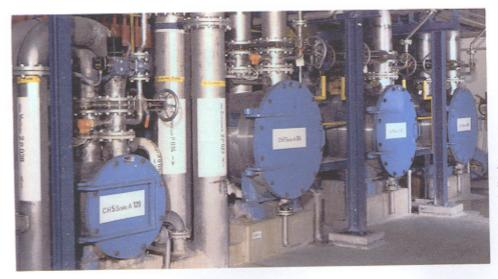
The horizontal design and screening efficiency of the CH enable multiple screens to operate in a relatively compact configuration. The hinged doors provide easy access to the screens and foil assemblies.
