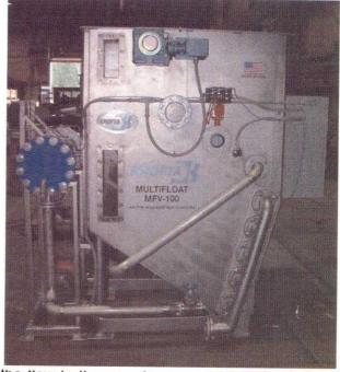
Should flow be shut-off to the unit, this ensures the flow to the recycle pump will not stop and cause damage to the pump. Floated materials are collected at the top of the FECs and directed towards the sludge collection rake assembly. The rake pushes the floated material over a simple beach design and deposits the material into a small sludge collection trough that is discharged by gravity.
