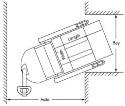
Aisle dimensions listed above assume the minimum bay width to be straddle OD plus 5" (2.5" on either side of straddle leg). Straddle OD is the load width plus 10". Track performance may vary due to application requirements and changes in model design.
