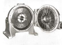
Hinged end housing—Plate access is a hinged end housing which contains the adjusting mechanism and sliding head assembly. Plates shown are one-piece design. Segmental overlap plates are also available.
