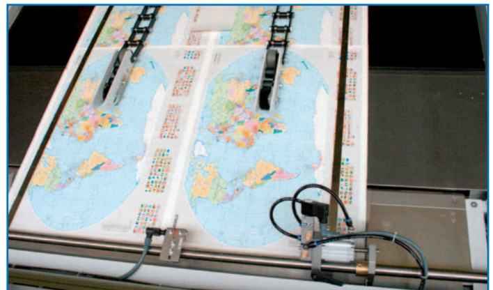
Suction-belt feeder for substrate sheets
