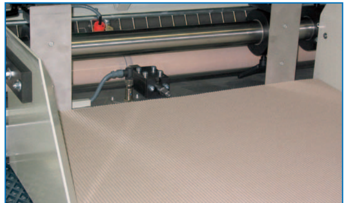
Suction-belt feeder for substrate sheets
