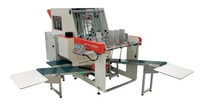
Automatic rotative grooving machine for board cases, supplied with a double feeder, grooving unit for "U" and "V" cuts and a double delivery unit.
