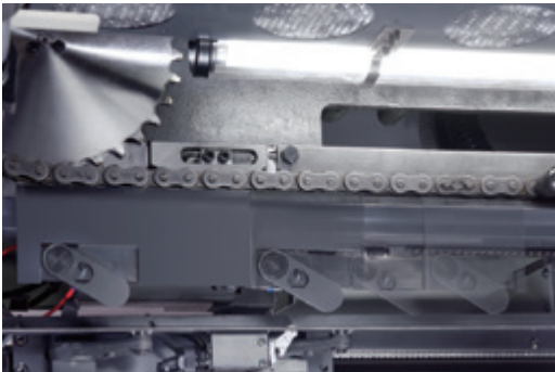
Side Jogger Linked to Sheet Size Sheet delivery is improved by the addition of a side jogger expansion/contraction function. Through linkage to the sheet size preset, the side jogger expands/contracts not only laterally but also along the top/bottom axis, improving sheet alignment performance with a variety of sheet sizes.
