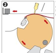
The squeegee moves down and printing starts at the top of the cylinder. The screen frame moves and the vacuum cylinder rotates
