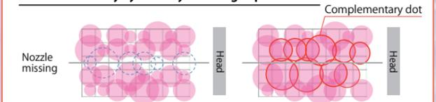
Fill the missing nozzles by enlarging the dots of the adjacent nozzles. (It gets missing nozzle stripes inconspicuous while printing by the Single-pass mode.)
