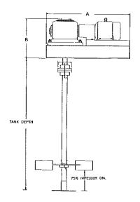
length and the rigid coupling length. A bottom shaft stabilizer is supplied with the MA-3 on installations in tanks six feet and deeper and other models at eight feet and deeper, to reduce side loading on the bearings. The stabilizer also protects the shaft and impeller when auxiliary equipment is carried inside the tanks during location moves.
