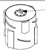
Lifting lug on the access cover should be in the up position as shown. The lifting lug is provided for shipping/in-plant handling only.
