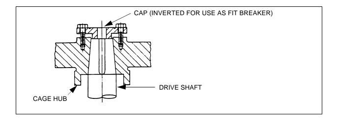
NOTE: The cap is made with a boss on the top side. This design permits the cap to be used as a fit breaker when removed and turned over.
