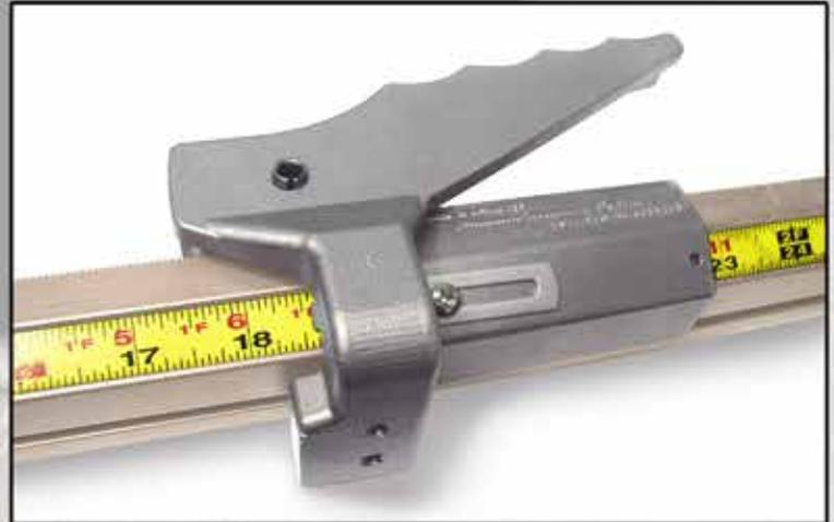
*Simply squeeze the handle on the Quick-Loc Stop System, slide it into position, and release it. The teeth on the stainless steel stop align themselves to the teeth on the rail to give you exactly the dimension you set. Once set into place, the stop cannot slip!*
