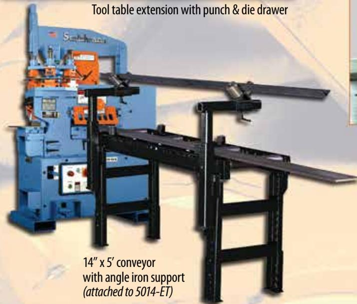
14" x 5' conveyor with angle iron support (attached to 5014-ET)
