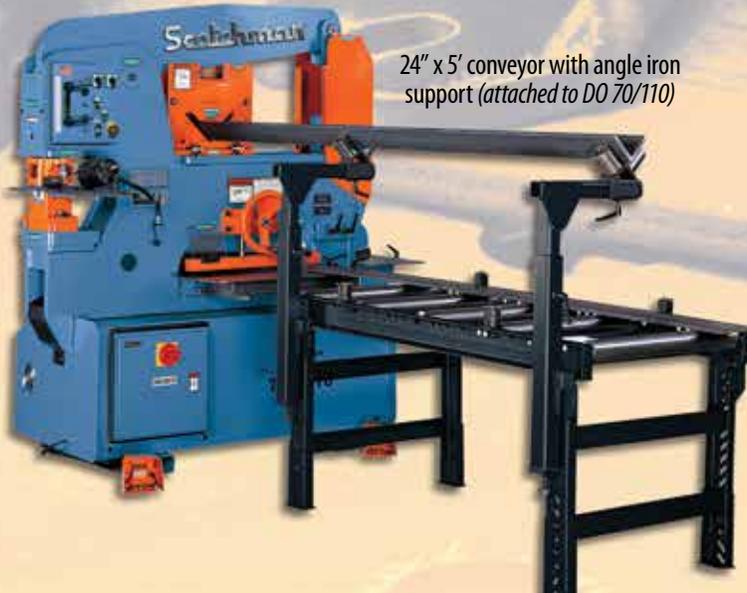
24" x 5' conveyor with angle iron support (attached to DO 70/110)
